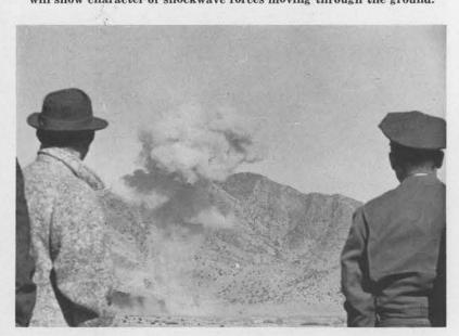
TOPPING OUT, the cloud towers over the Manzanos, but there will be no "fallout" because it is a non-nuclear test, set off in Sandia's Backyard Bikini to provide information to be used in planning peaceful applications of nuclear blasts, such as mining and harbor work. The work is performed under the direction of D. G. Palmer (5112), with cooperation of many Sandia groups.
